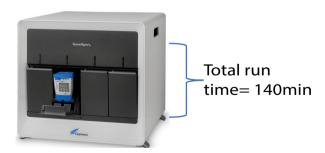
Load the cartridge in the GeneXpert machine and start the run
