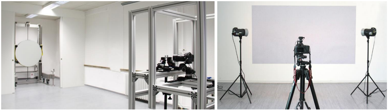
Fig. 1 Setup of the single-mirror coincident schlieren system (left) and the BOS system (right) at the Department of Building Physics at the Bauhaus-University Weimar
