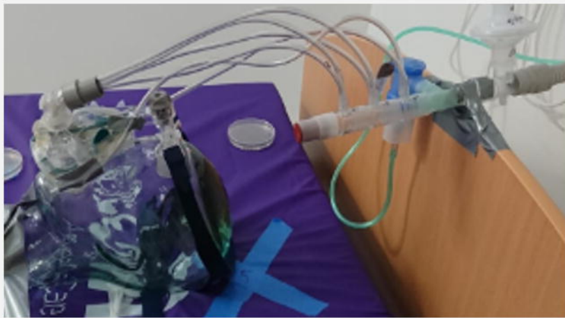
C. Leak circuit attached to glass head
