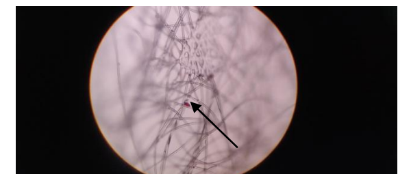
Photo 9: Stain observed in the inner layer of triple layer surgical mask (100x)
