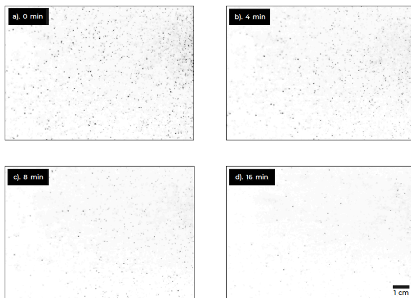
Figure 2 – Laser-illuminated aerosol droplets at different times after initial spraying. Initially (a), droplets have a maximum sedimentation velocity of about 2 cm/sec, corresponding to droplets of about 25 \mu\text{m} in diameter. In the 16 min frame (d), the fastest moving droplet has a sedimentation velocity of at most 1 mm/sec, corresponding to a droplet of about 4-5 \mu\text{m} in diameter.
