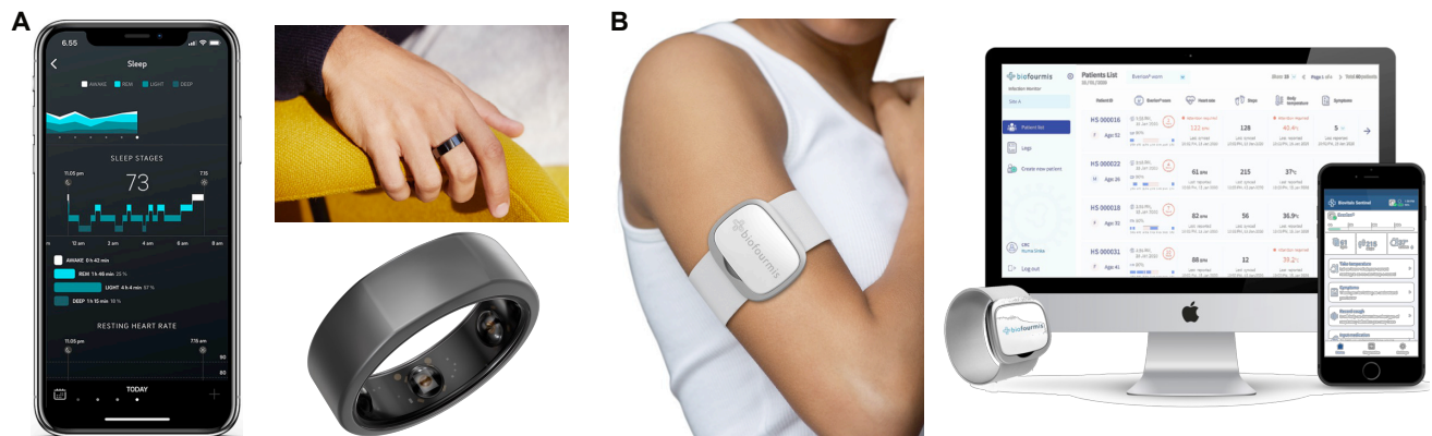
Figure 1. Examples of wearable technology. A) the Oura Smart Ring sensor and an image of the app utilized to collect and display physiological data collected using the sensor. B) the Everion system by Biofourmis. The system is used to collect data such as heart rate, respiratory rate, and oxygen saturation. Images reproduced with permission by the manufacturers.
