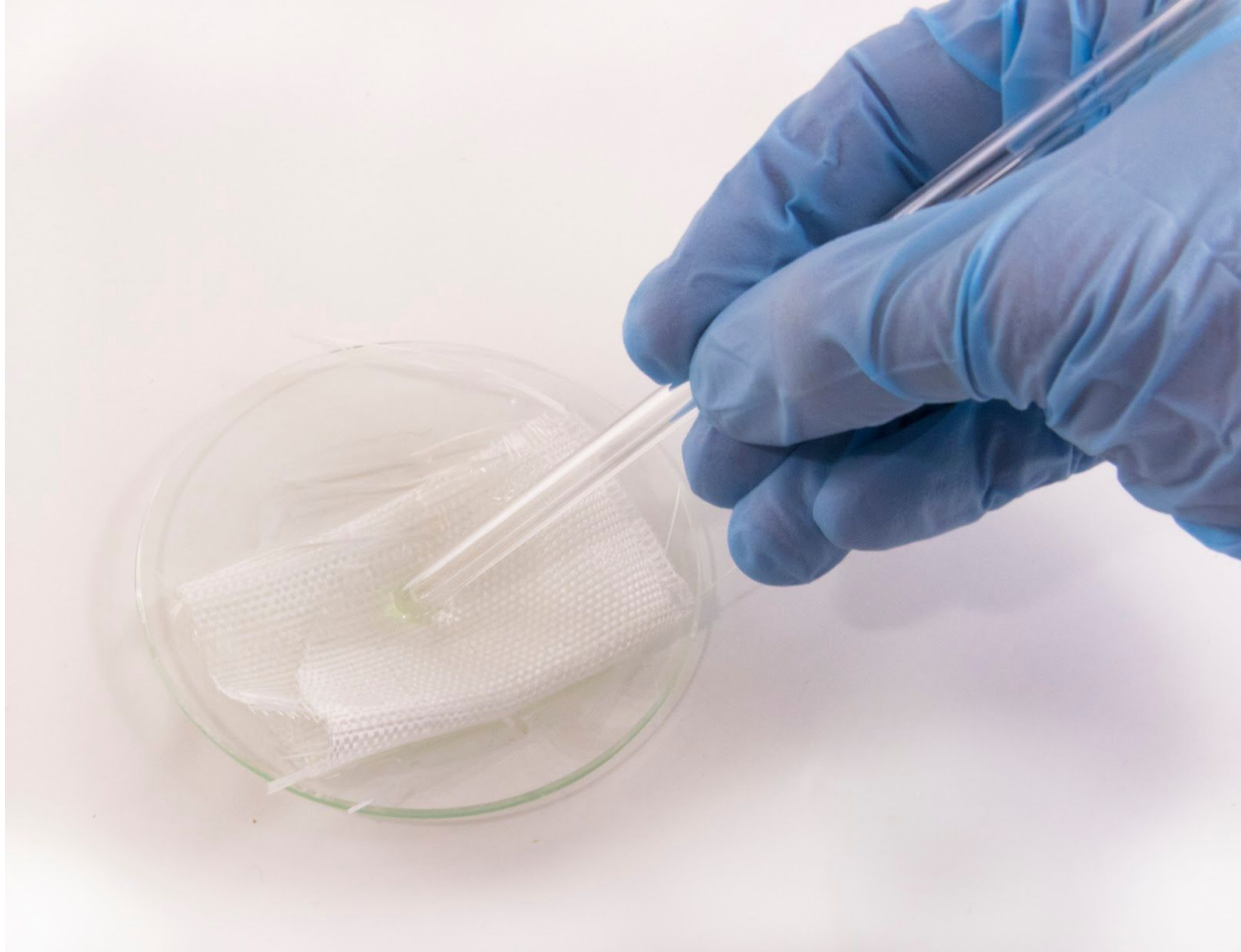
Fig. 6. A woven fiberglass cloth swatch, used as a nonreactive fiber matrix to increase the rate of vaporization, placed into a dish of hydrogen peroxide solution. The action of soaking the cloth in hydrogen peroxide solution by use of a stir rod is depicted.
