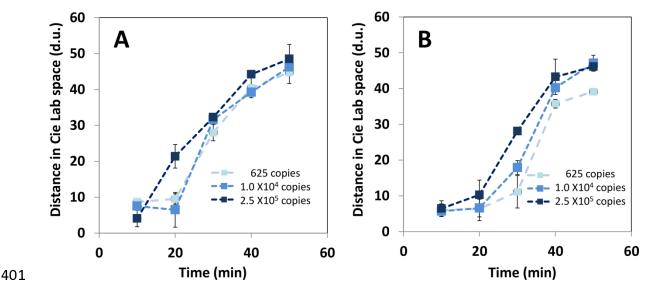
Figure 5. Time progression of the distance in color with respect to negative controls (red color) in the CIELab space for positive SARS-CoV-2 samples containing 625 (light blue,  $\blacksquare$ ),  $1 \times 10^4$  (medium blue,  $\blacksquare$ ), and  $2.5 \times 10^6$  (dark blue,  $\blacksquare$ ) copies of synthetic of SARS-CoV-2 nucleic acids. Results obtained in experiments using (A) primer set α, and (B) primer set β.
