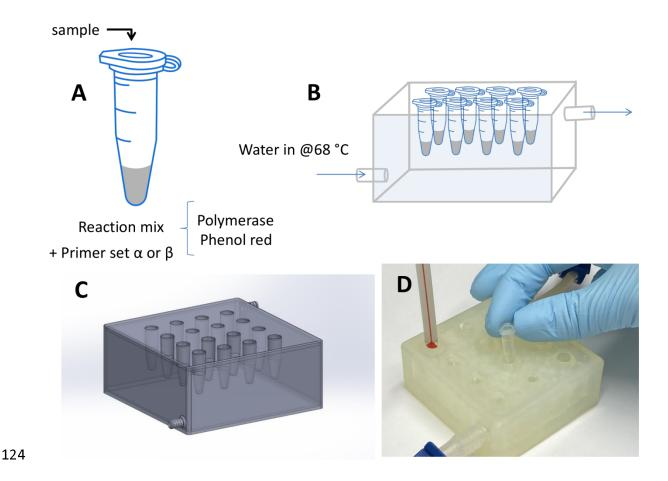
**Figure 1. Experimental setup.** (A) Commercial 200 microliter Eppendorf PCR tubes, and (B) a 3D-printed incubator were used in amplification experiments of samples containing synthetic SARS-CoV-2 nucleic acid material. (C) 3D CAD model of the LAMP reaction incubator. (D) Actual image of the Eppendorf tube incubator connected to a conventional water circulator.
