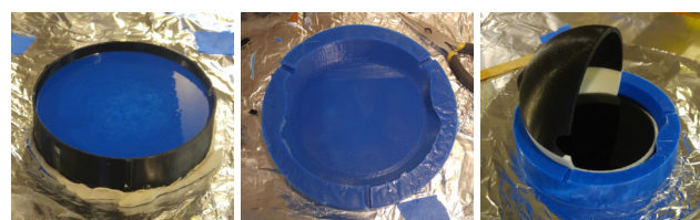
Figure 9. On the left, making a mold to make the face screen. In the middle, the completed mold for the face screen, which is used to mold the translucent front screen. On the right, the translucent front screen being molded into a prototype 3D printed model of the head. The material being used is a clear urethane with black colorant added.
