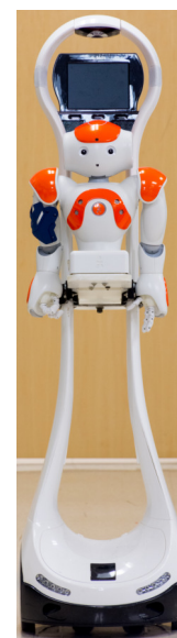
Figure 1. The first version of our social robot on a telepresence system, Flo, composed of a Nao robot attached to a VGo telepresence robot.
