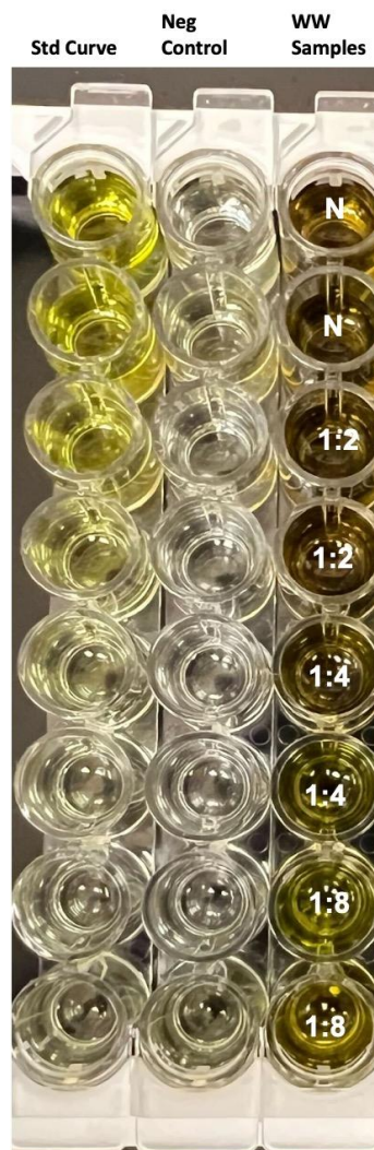
Figure 2b. Representative ELISA plate assay for concentrated wastewater evaluated for total IgA by ELISA. The first column of wells in the plate contains a standard reference dilution series. The second column contains the negative control. Wastewater samples are labeled by row as Neat or by dilution factor.
