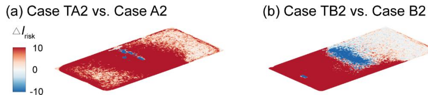
FIG. 17. Comparison of the I_{\text{risk}} map at the breathing level between the simulation cases with and without consideration of thermal effect for the infector (a) in the front and (b) in the middle of the classroom with the air cleaner near the HUUV. The \Delta I_{\text{risk}} is defined as the I_{\text{risk}} of Case TA2 subtracted by that of Case A2 for (a) and the I_{\text{risk}} of Case TB2 subtracted by that of Case B2 for (b).
