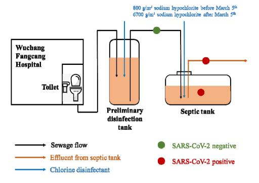
Figure 1. Schematic disinfection process of septic tanks of Wuchang Fangcang
